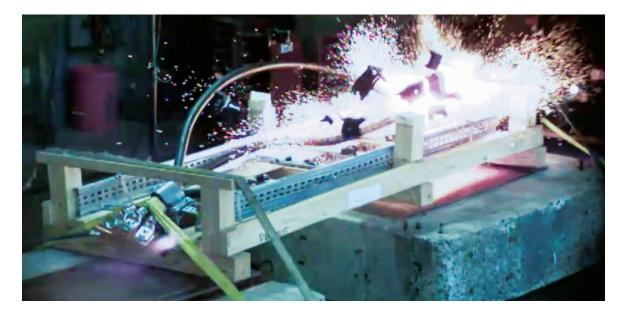
To suggest that a strap banding system is not suitable for short circuit rated installations is incorrect and is out dated information. The cable system designer must make sure that the fault levels have been accurately calculated and then specify a fixing system which meets that requirement and complies fully to IEC 61914:2015
